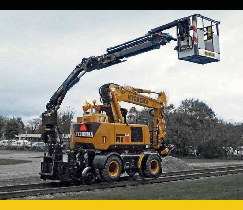
Purpose-build, detachable crane with man basket for railway construction and maintenance. Can be mounted on the Hydrema range of MX RAIL excavators.
