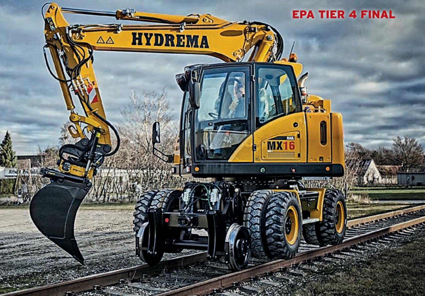
**Specially designed compact excavator in the 19 ton class for railway work with focus on great stability, high performance and flexibility.**
