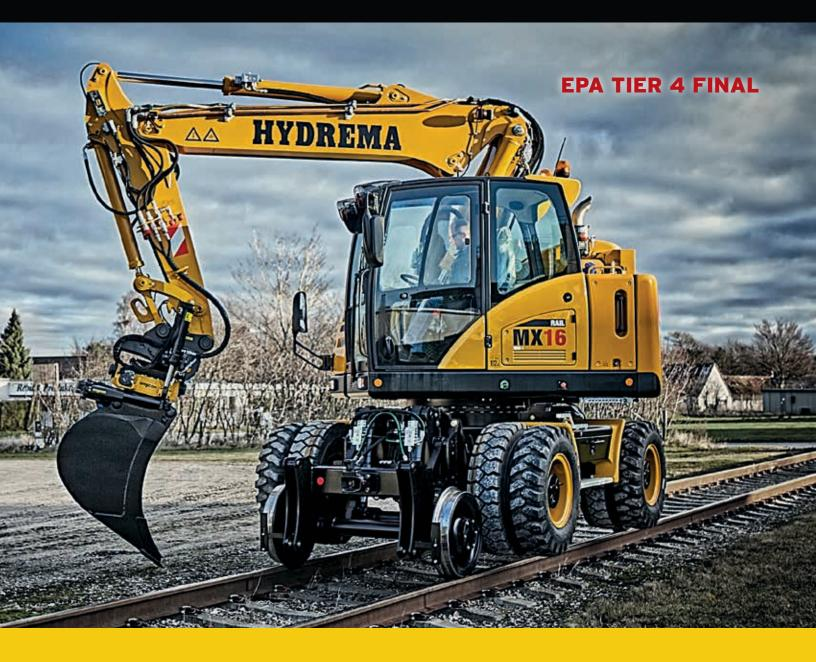
Specially designed compact excavator in the 19 ton class for railway work with focus on great stability, high performance and flexibility.
